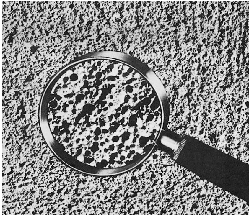
The magnified portion of this insulating cellular concrete shows the remarkable size and shape uniformity of the tiny non-connecting air cells.
